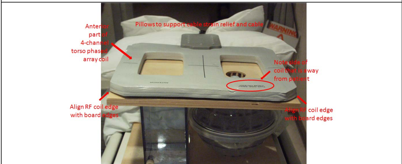
Figure A.7. Place the anterior part of the phased array RF coil on top of the top birch board. Also, make sure that this top assembly of coil and board align with the bottom assembly of board and coil. Use multiple pillows (or equivalent, but pillows seem to be best!) to support the cable and the extension of
