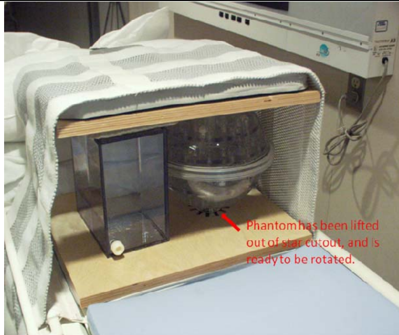
Figure B.2(a). Without allowing the lower birch board to move, lift the spherical phantom out of the star cutout of the birch board. Rotate the spherical phantom by 90 degrees and reset the phantom in the star cutout.
