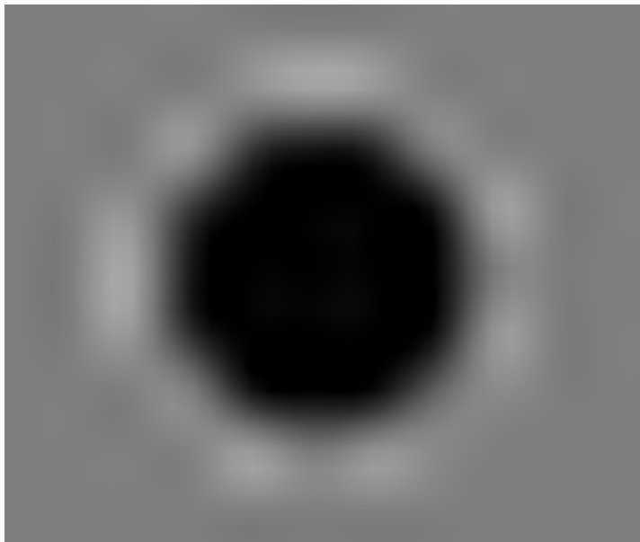
(a) Zoomed view of the smallest hot sphere (sphere 1). Slight spatial distortions and slight ringing artifacts are apparent. A complex ringing perpendicular to the sphere wall and a horizontal/vertical streaking has been observed on some displays.
