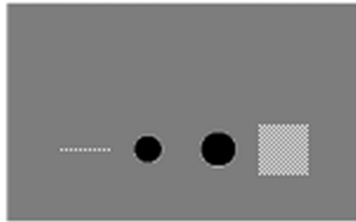
(d) Coronal view of the PET DRO showing the 2D test pattern in slice 40 (left) as well as the 3D cubic test pattern (right).
