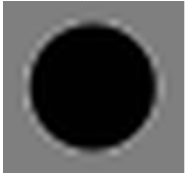
(b) Zoomed view of the largest hot sphere (sphere 6). Ringing artifacts are apparent outside the wall of the sphere, and the top and bottom of the sphere wall appear to be truncated. A complex ringing perpendicular to the sphere wall has been observed on some displays.
