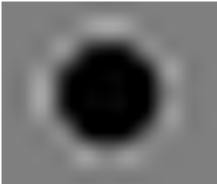
(a) Zoomed view of the smallest hot sphere (sphere 1). Slight spacial distortions and slight ringing artifacts are apparent. A complex ringing perpendicular to the sphere wall and a horizontal/vertical streaking has been observed on some displays.
