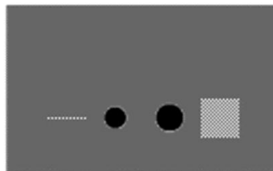
Coronal view of the PET DRO showing the 2D test pattern in slice 40 (left) as well as the 3D cubic test pattern (right)
