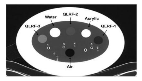
Figure 1. COPDGene®2 test object with cylindrical foam density standards and acrylic tubes mimicking airway wall and lumen. Densities are indicted below in Table 1.
