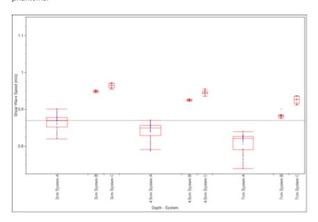
**Figure 2.** A. quantile plot showing statistically signficant differences among three different ultrasound systems (A,B & C) measuring shear wave speed over three depths (3, 4.5 & 7cm) on pilot QIBA phantoms.
