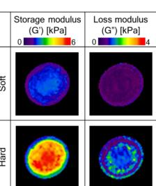
Storage and loss modulus maps of the MRE phantoms with different viscoelasticity
