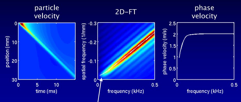
Maximum in 2D-FT along temporal frequency deviates from constant velocity at low frequencies
