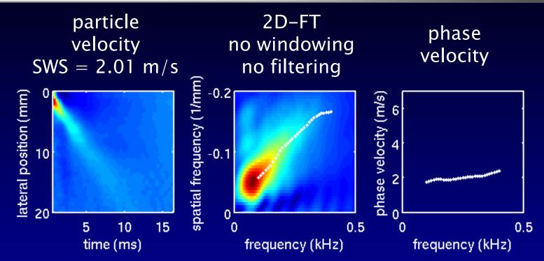
phase velocity  $c(\omega) = \omega/k$
