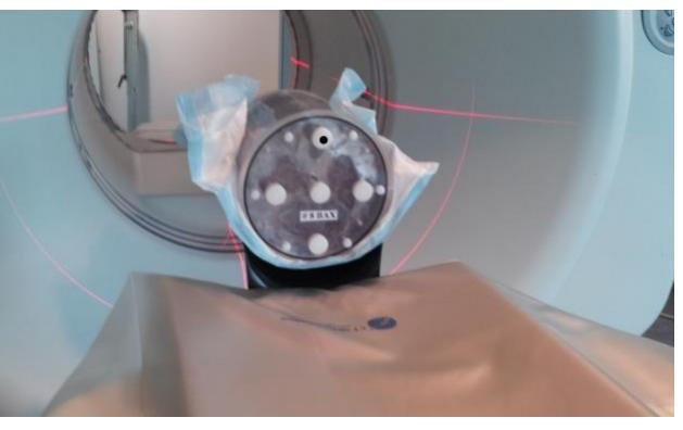
2315 **Figure 12.** Positioning of Hoffman Brain Phantom in scanner.
