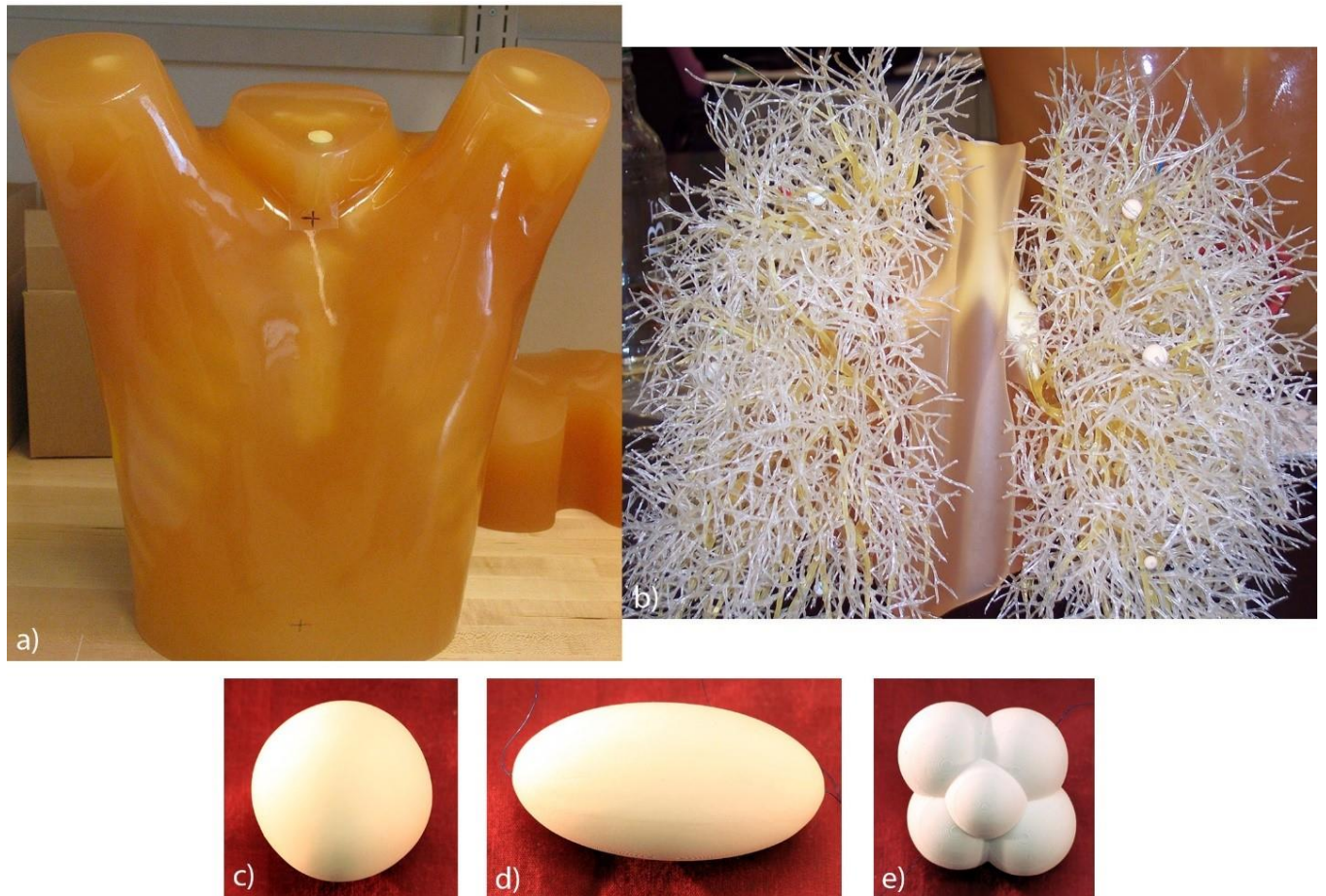
Fig. 1: (a) Anthropomorphic thorax phantom, (b) vascular insert, and the three nodule shapes: c) spherical, (d) elliptical, (e) lobulated used for conformance testing of software tools and radiologists.
