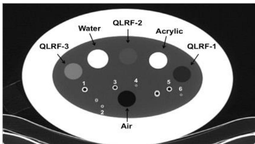
Figure 1. COPDGene®2 test object with cylindrical foam density standards and acrylic tubes mimicking airway wall and lumen. Densities are indicated below in Table 1.
