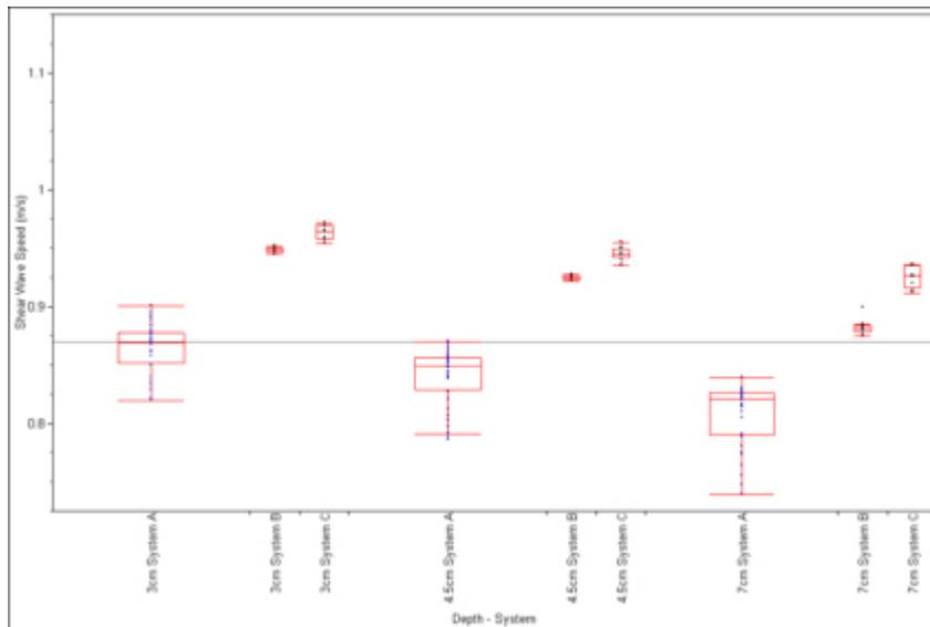
**Figure 2.** A quantile plot showing statistically significant differences among three different ultrasound systems (A, B & C) measuring shear wave speed over three depths (3, 4.5 & 7cm) on pilot QIBA phantoms.
