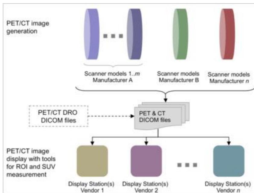
**Figure 1.** Data flow for PET/CT DICOM images. The proposed role of the PET/CT digital reference object (DRO) as a reference standard is also shown.
