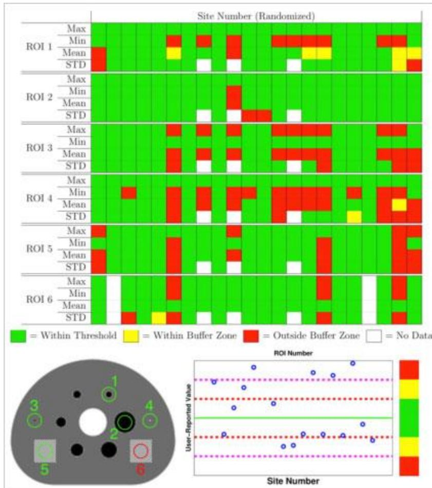
**Figure 2.** Top: Results from user-reported SUV values from the PET/CT DRO. Each column represents a single site/system and each row corresponds to a metric from one of the six ROIs indicated. Bottom: ROIs overlaid on the primary slice of the PET component of the DRO and an illustration of the threshold definitions for one ROI metric.
