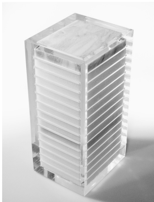
Figure 1. Perspex box containing 15 compartments with pieces of foam, representative of lung tissue.
