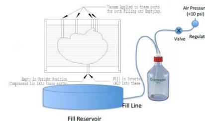
Phantom fill procedure uses low pressure air to push the radioactive solution into the main brain compartment using 8 fill holes. Vent holes allow for air to escape easily during filling.
