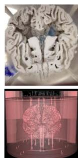
Phantom assembly (top) and a rendered CT scan of assembled phantom (bottom).
