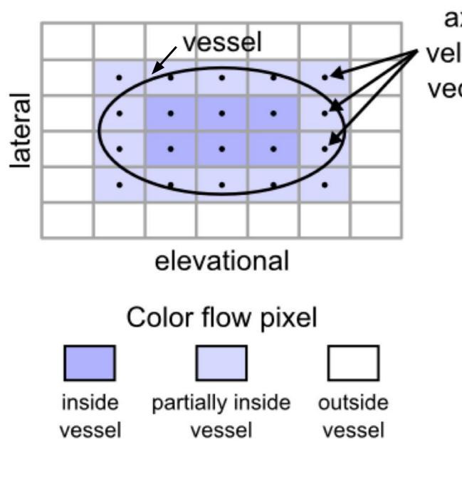
Partial volume effect in 3D volume flow measurement. Three types of color flow pixels exist. Color flow pixels inside the vessel correspond to 100% blood, those outside the vessel correspond to 0% blood, and those partially inside the vessel correspond to values between 0% and 100% blood. Color flow power is directly proportional to the amount of blood in each voxel and can therefore be used to correct the partial volume effect.
