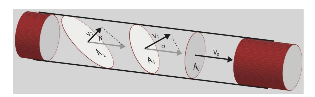
3D volume flow (Q) is computed by multiplying blood flow velocity ( $v_n$ ), as measured by color flow, by the surface area of the intersected lumen ( $A_n$ ). Given that Q =  $A_0 \times v_0 = A_1 \times v_1 = A_2 \times v_2$ , 3D volume flow is independent of angle. Specifically,  $A_n = A_0 / \cos(\alpha_n)$  and  $v_n = v_0 \times \cos(\alpha_n)$ , therefore, the cosine factor cancels when A is multiplied by v.
