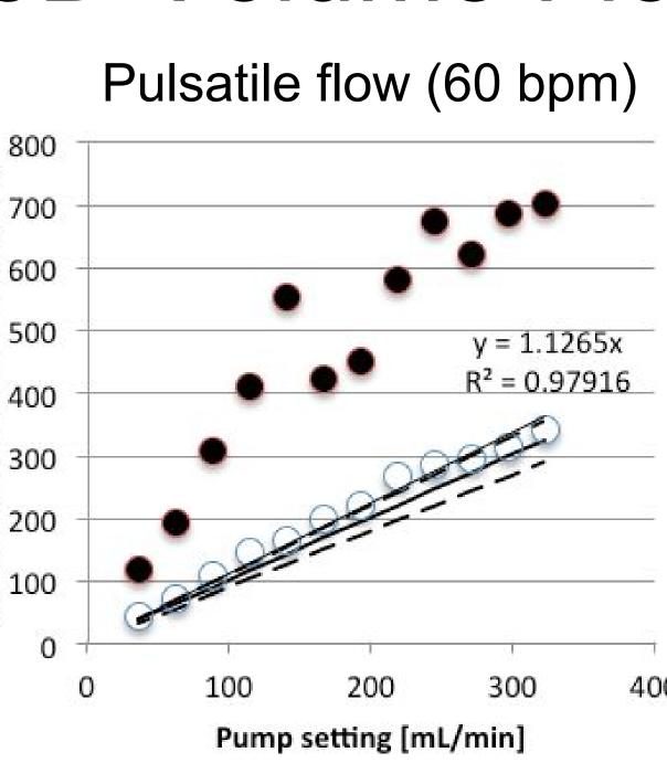
Phantom study results for 78 to 696 mL/min (left) and 43 to 341 mL/min (right) show partial volume corrected (○) and not partial volume corrected (●) data. The thin solid line is the linear regression fit and the thick solid line represents true flow with ±10% intervals (dashed lines). Nominal lumen diameter is 5 mm.
