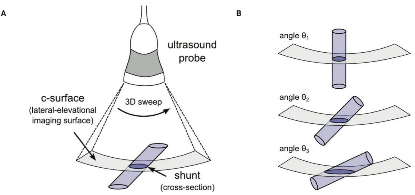
Illustration of (A) imaging geometry required for 3D volume flow measurement. Probe is oriented such that the lumen intersects the c-surface (lateral-elevational surface) in cross section. (B) Angle of c-surface intersection is an independent variable such that circular ( $\theta_1$ ) and ellipsoidal ( $\theta_2$  and  $\theta_3$ ) geometries all yield identical volume flow estimates without the need for any angle correction.
