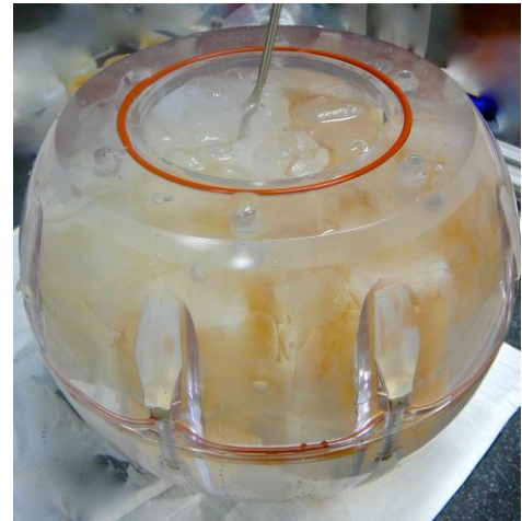
Figure 1. Phantom after being in the refrigerator overnight. Add more crushed ice to displace any melted water in order to maintain a 0°C bath.
