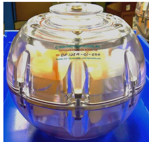
Figure 2. Assembled phantom. Secondary fill ports can be used to eliminate residual air bubbles.
