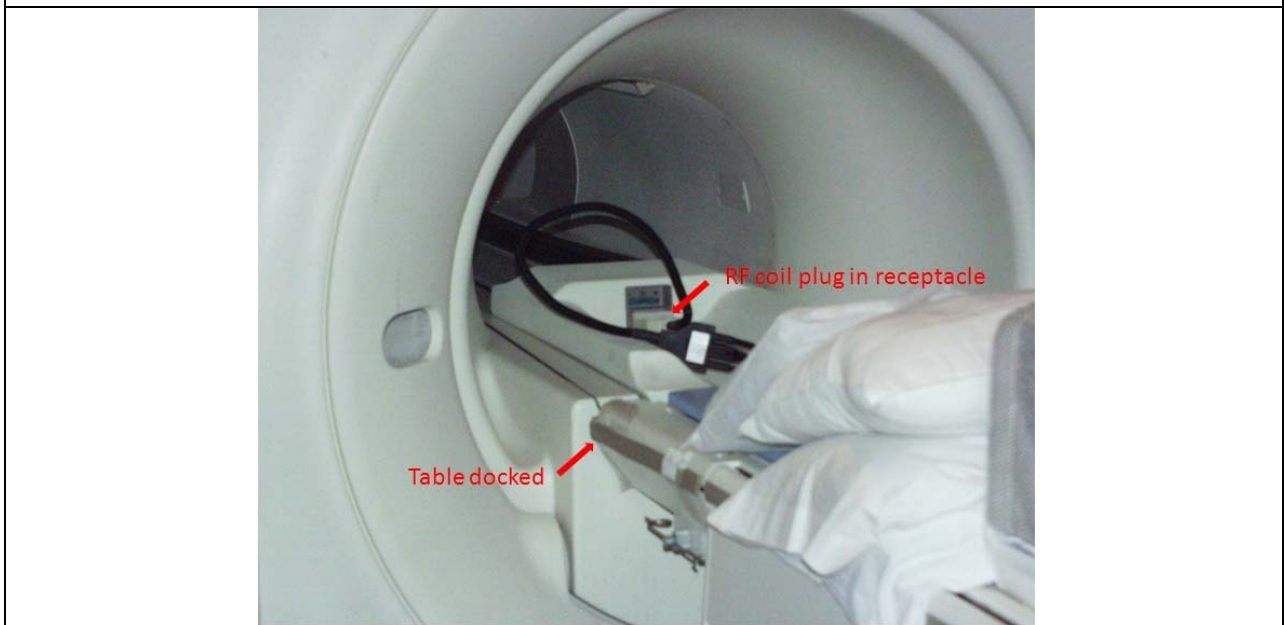
Figure A.11. Move the patient table with the final phantom assembly into the magnet room. Dock the patient table to the magnet, and insert the coil plug into the lower receptacle.
