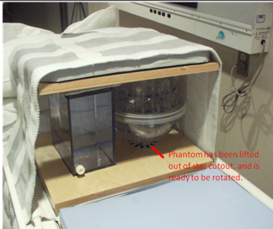
Figure B.2(a). Without allowing the lower birch board to move, lift the spherical phantom out of the star cutout of the birch board. Rotate the spherical phantom by 90 degrees and reset the phantom in the star cutout.
