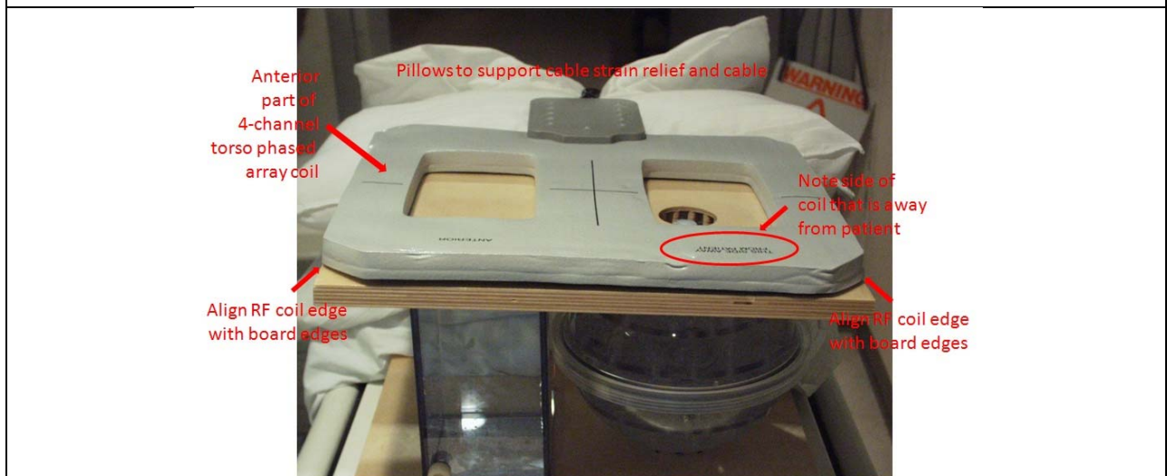
Figure A.7. Place the anterior part of the phased array RF coil on top of the top birch board. Also, make sure that this top assembly of coil and board align with the bottom assembly of board and coil. Use multiple pillows (or equivalent, but pillows seem to be best!) to support the cable and the extension of the top part of the phase array RF coil. The pillows will support the weight of the cable and cable strain relief, and will help to stabilize the top part of the RF coil on the birch board.
