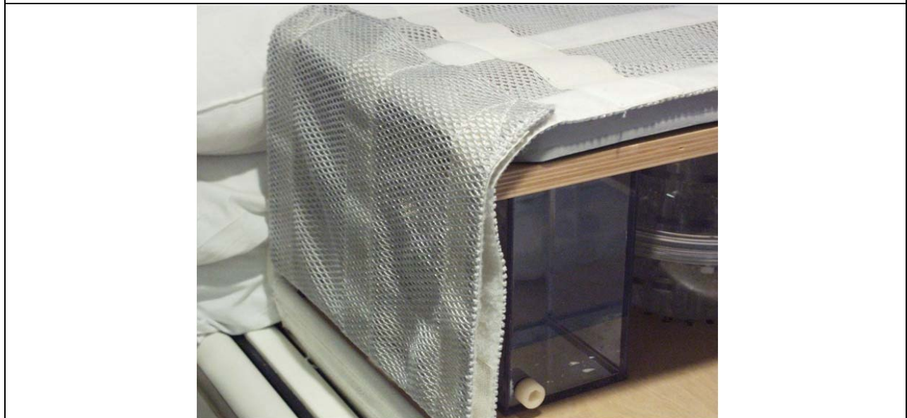
Figure A.9. Wrap the patient strap tightly around the total assembly. From the left side of the table, the strap should be carried over the assembly, carried down and put through the plastic ring on the right side of the table, and then pulled down. Prior to Velcro-ing the patient strap to itself along the top side, adjust the top assembly consisting of coil and birch board so that they are horizontal (parallel to the table), and also are aligned with the bottom assembly. There should be minimal pull down of the top assembly on either side.
