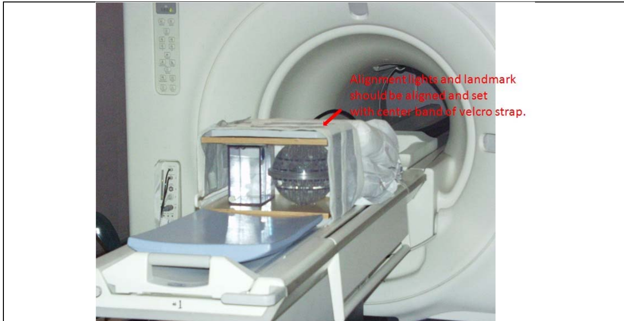
Figure A.12. Turn on the alignment lights, and move the table such that the assembly is bisected by the alignment lights. Make final adjustments of the assembly so that the alignment lights bisect the assembly both in the superior/inferior direction, AND the right/left direction. The alignment lights help to show the presence of poor alignment of the top and bottom parts of the total assembly. Set the landmark, and hit the Advance to Scan button to move the total assembly into the center of the magnet. After completing the protocol, bring the patient table to the “Home” position.
