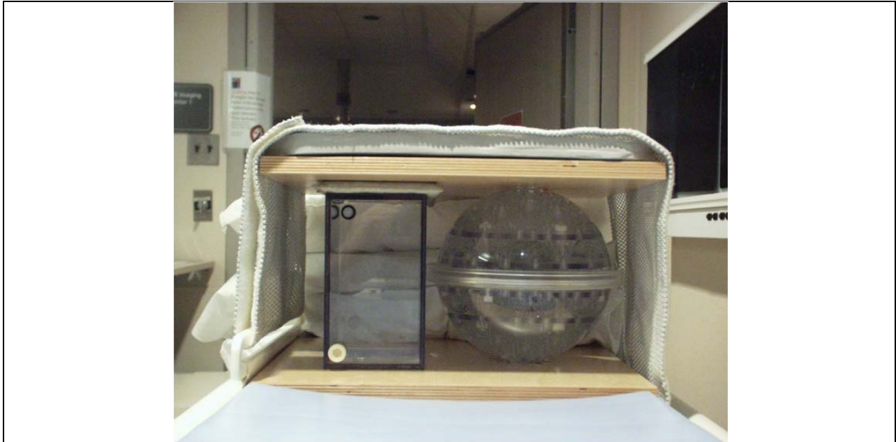
Figure A.10. Release the strap to adjust the top birch board and RF coil and achieve a horizontal orientation and alignment of the top assembly with the bottom assembly. Also, the patient strap should not be so tight as to cause the RF coil to flex. The flex will invariably cause a gap to form between the birch board and the RF coil. The gap will cause the RF coil to pick up less signal from the phantom, and hence should be minimized.
