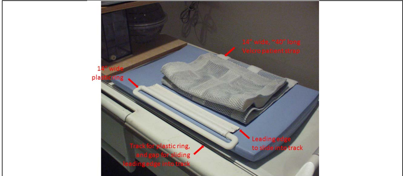
Figure A.8. On the patient table of the GE system, slide the wide (about 14" long) plastic ring assembly into the track along the left side of the table. On the right side of the table, slide the broad patient strap into the track. This patient strap is approximately 40" long and will serve to secure the total assembly of coil, birch board, spherical phantom and cuboid and make it a rigid structure.
